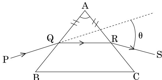
A ray PQ incident on the refracting face BA is refracted in the prism BAC as shown in the figure and emerges from the other refracting face AC as RS such that  $AQ = AR$ . If the angle of prism  $A = 60^\circ$  and refractive index of material of prism is  $\sqrt{3}$ , calculate angle  $\theta$ .
