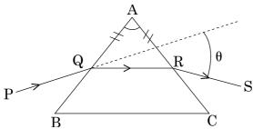
A ray PQ incident on the refracting face BA is refracted in the prism BAC as shown in the figure and emerges from the other refracting face AC as RS such that AQ=AR. If the angle of prism  $A=60^\circ$  and refractive index of material of prism is  $\sqrt{3}$ , calculate angle  $\theta$ .
